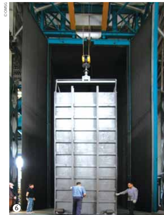
Figure 6: A large container being placed inside the shotblasting machine.
