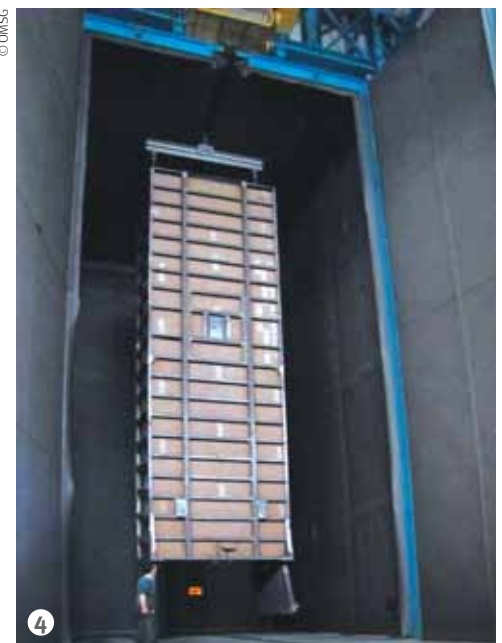
Figure 4: A container waiting to be shotblasted.
