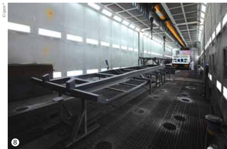
Figure 8: The large oven chamber has three workstations.
