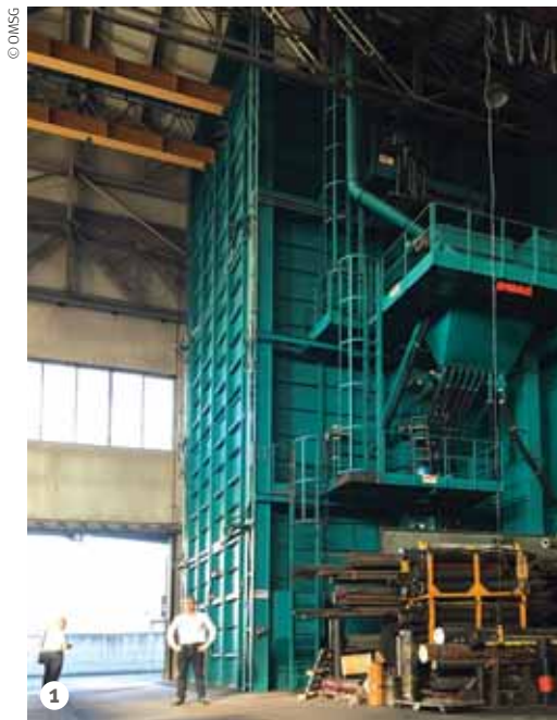
Figure 1: The huge shotblasting machine provided by OMSG.
