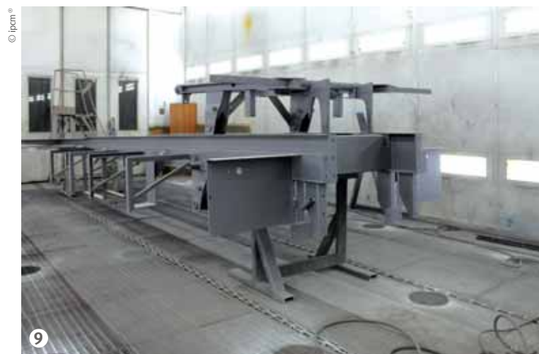
Figure 9: A shotblasted frame ready to be coated.
